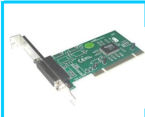
PCI-08 PCI To Parallel ASK
