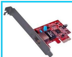
PCI-11 PCI-E To Lan Card (10/100/1000) ASK
