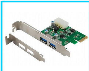
PCI-10E(LP) PCI-E To USB 3.0 Card (2Port) w/ Low-Profile ASK
